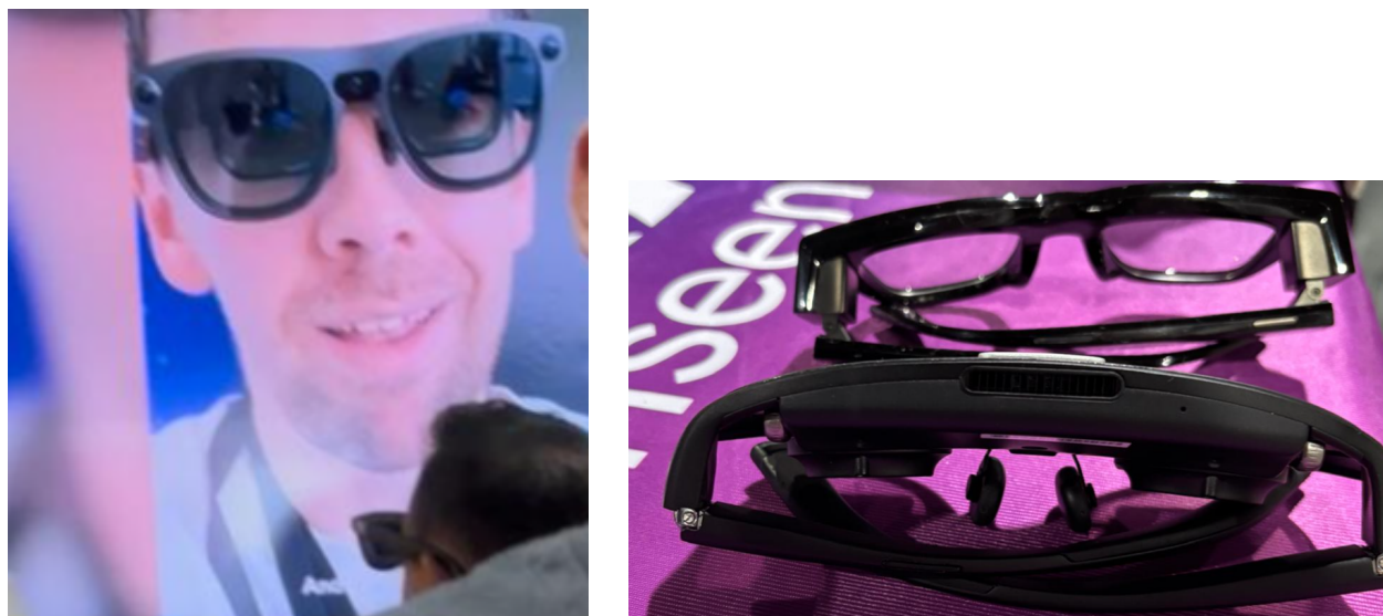
Figure 3: XREAL Aura, worn on the floor (left). Right — top, Meta Ray-Ban Display; bottom, Unseen Reality URXR One. The optical display is invisible in Category 1, but in Category 2 it is a miniaturized headset with its own lenses, showing the world through front-facing see-through cameras.
