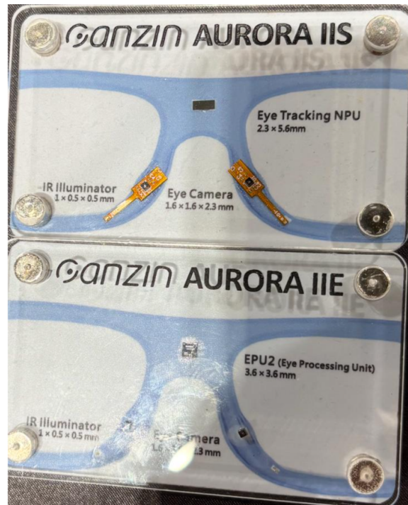
Figure 7: Ganzin's Aurora IIS and Aurora IIE eye-tracking reference modules.
