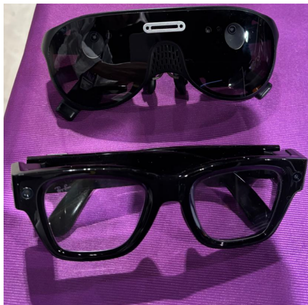
Figure 1: The AWE 2026 floor in Long Beach (left). Right — two near-identical-size frames from opposite categories: top, the Unseen Reality URXR One (Category 2: 6DoF, tethered display, video passthrough); bottom, the Meta Ray-Ban Display (Category 1: 0DoF/3DoF HUD, wireless, fully transparent).
